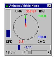
This window provides a graphical representation of the vessel's navigation parameters with comparisons of the Vehicle's Heading (green), the Vehicle's Course Made Good (blue), and the Bearing of the Survey Line (red).
